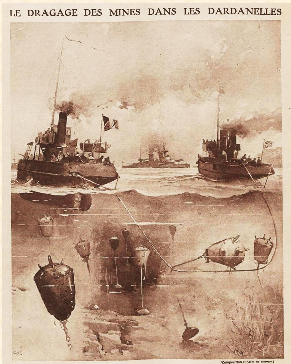
French and British trawlers minesweeping in March 1915 during the Allied naval campaign in Turkey's Dardanelles Strait. They are seen using a technique developed with trawlers from Grimsby in 1908. Some of the British trawlers in the Dardanelles were also from Grimsby. Turkey had closed the Strait to starve Russia of supplies from the Mediterranean via the Black Sea. The trawlers cleared channels to enable British and French warships to force their way through to Gallipoli. (Illustration by Paul Carrey; published on 4 April 1915 in edition 71 of Le Miroir, the Sunday supplement to the French daily newspaper Le Petit Parisien; Commons.Wikimedia.org )
